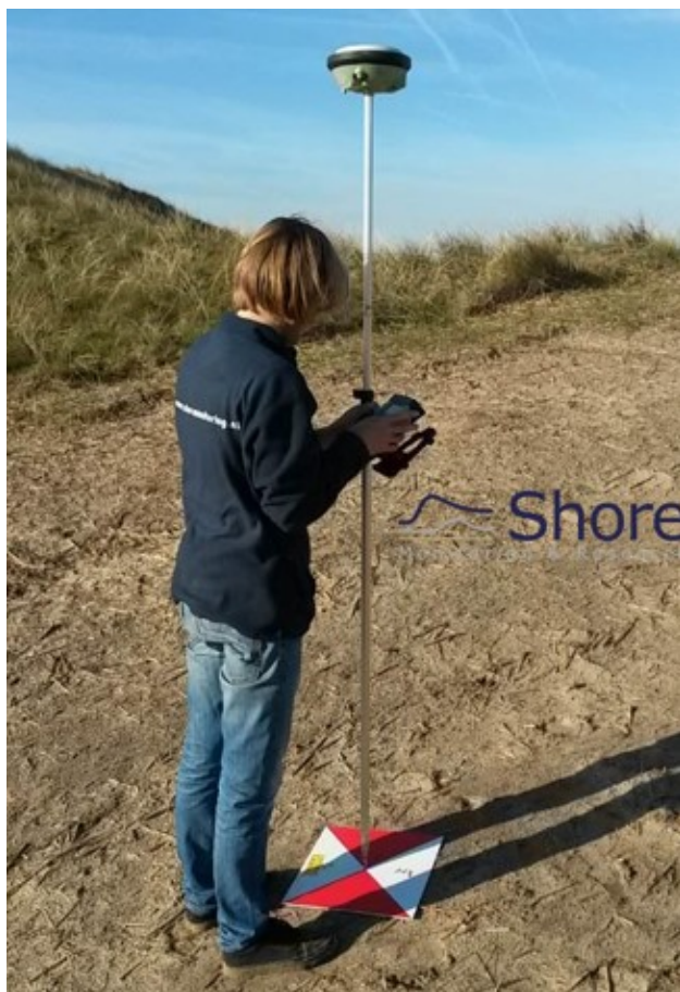
Figure 4.4: Typical rover set-up
