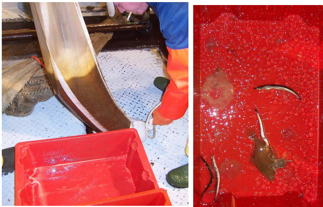
Plate 3. MIK sampler cod end during sample recovery (left) and plankton sample before sorting.
