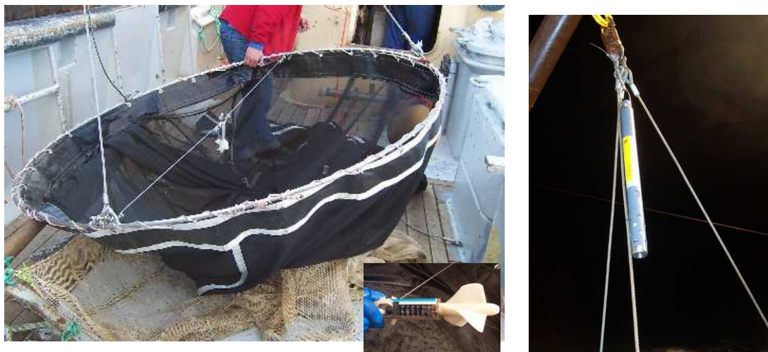
Plate 2. MTK method sampler (right) and water quality (WQ) data logger (left) used in the pelagic survey. The sampler is fitted with a central flow meter (see insert picture for a close up view) and is shown on the vessel's deck. The WQ data logger is shown fitted to the MTK sampler bridle lines.
