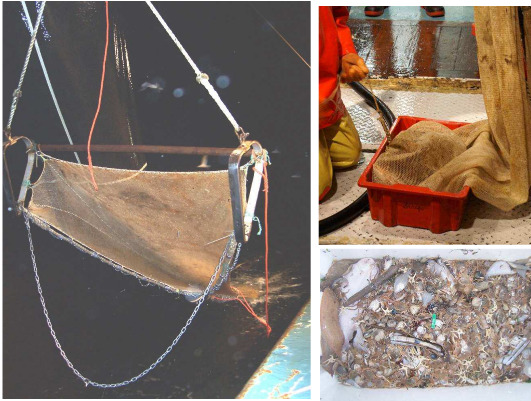
Plate 1. Beam trawl used in the demersal survey. The sampler is shown fully rigged ready to be deployed from the side beam of the survey vessel (left). Detail of the cod end during recovery of the sample after a demersal tow (top right) and typical unsorted catch (bottom right).
