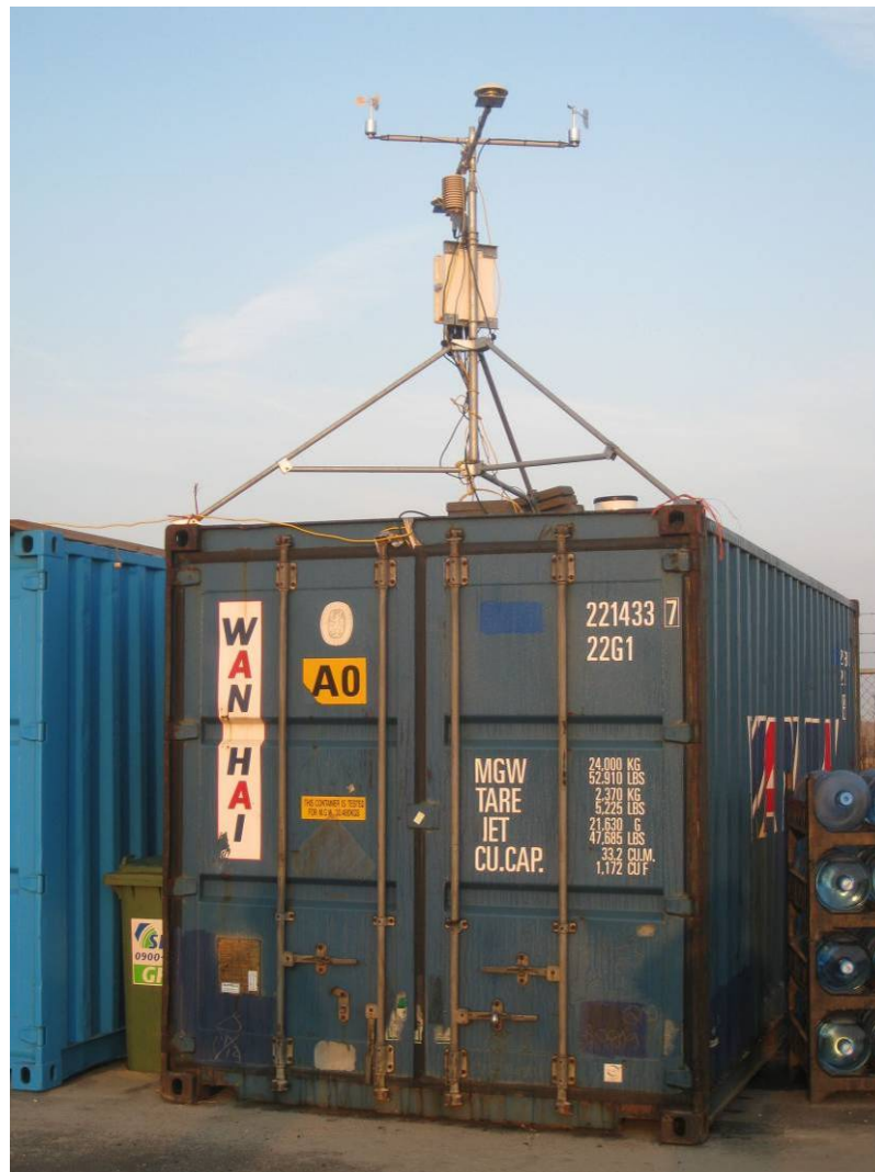
Figure 6.3 The land-based meteo system, placed on top of a cotaniner in the Maasvlakte area (see Figure 6.1 for the location).
