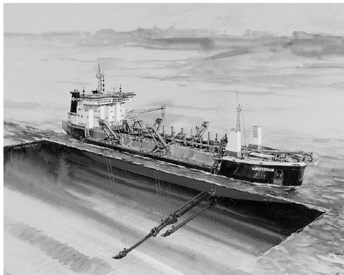
Figure 1 Illustration of a trailing suction hopper dredger in operation. (Image taken from [13].)
