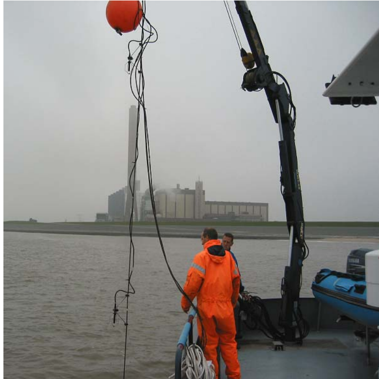
Figure 9 Example deployment of a chain with two hydrophones and a surface buoy.
